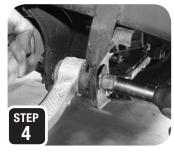
bolts, then loosen and remove both bolts. **STEP 5:** Lower the jack and remove the strut.
