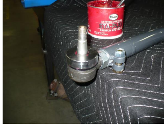
Figure 5. Bushing and cap installed
