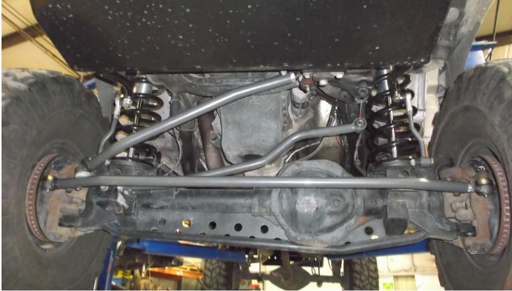
Figure 18. 8567-01 drag link shown with bend forward/flat
