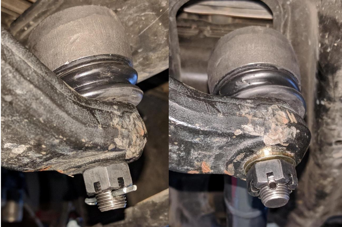
Figure 23 and 24. Washer used under castle nut in order for cotter pin to engage castle nut
