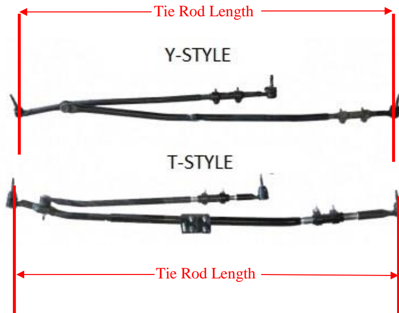
Figure 1. How to measure tie rod length
