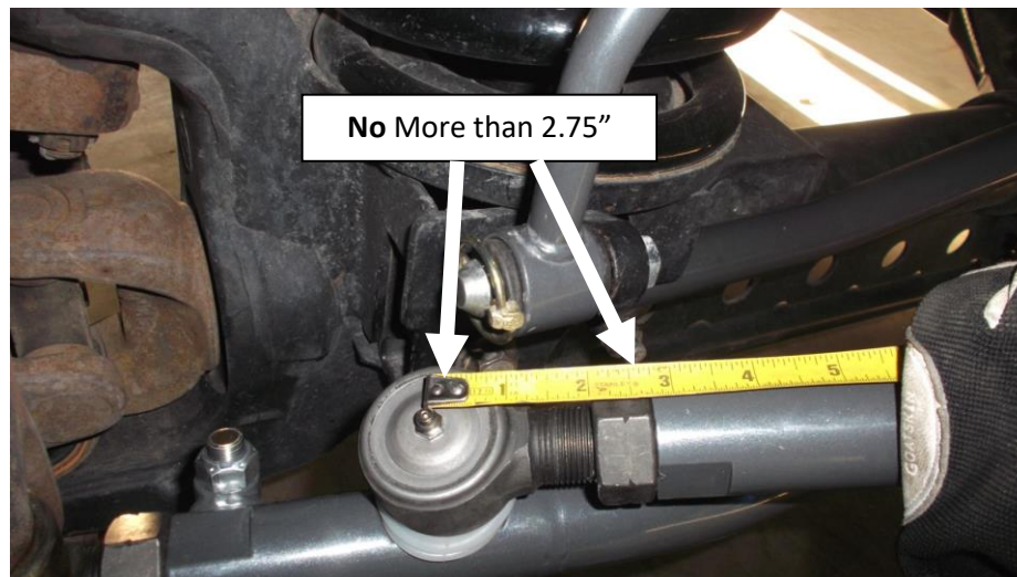
Figure 19. Tie rod end adjusted MAX 2.75" out
