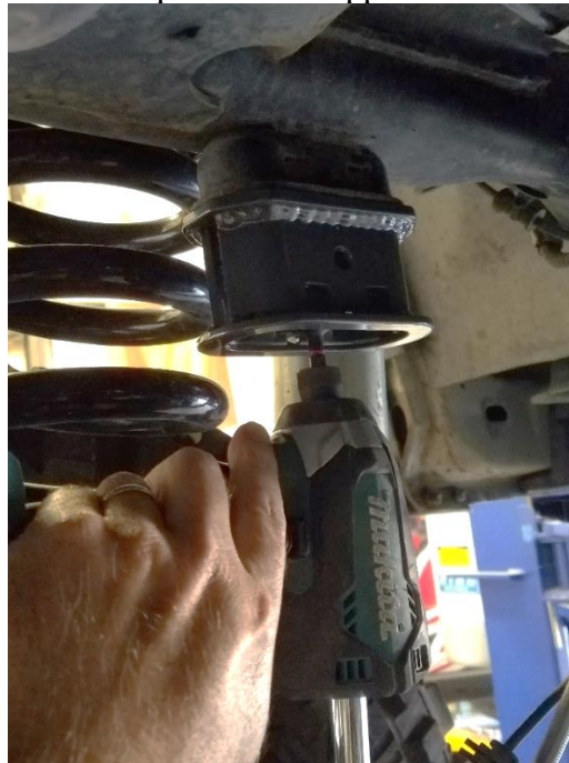
Figure 4. Installing self tapping screw.
