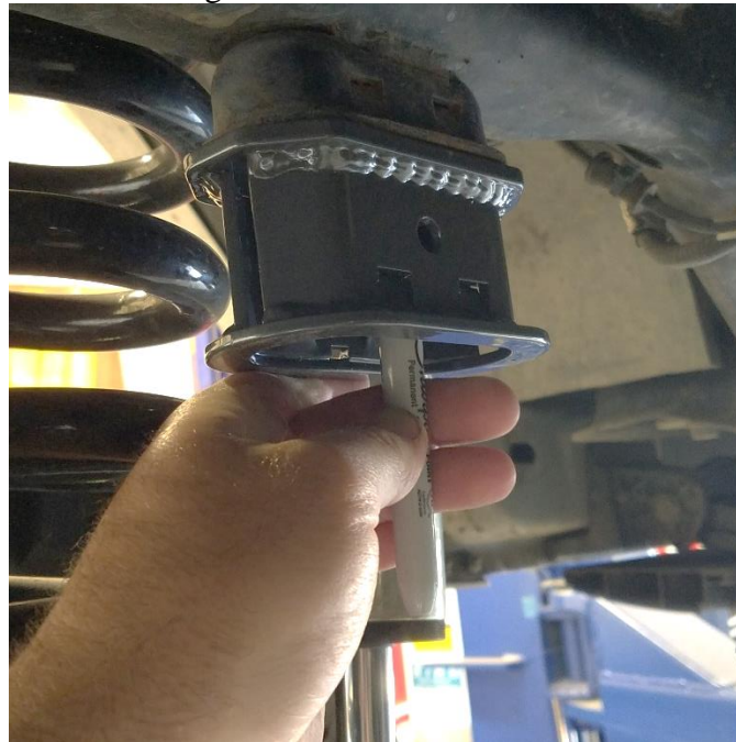
Figure 2. Marking the location for the hole.
