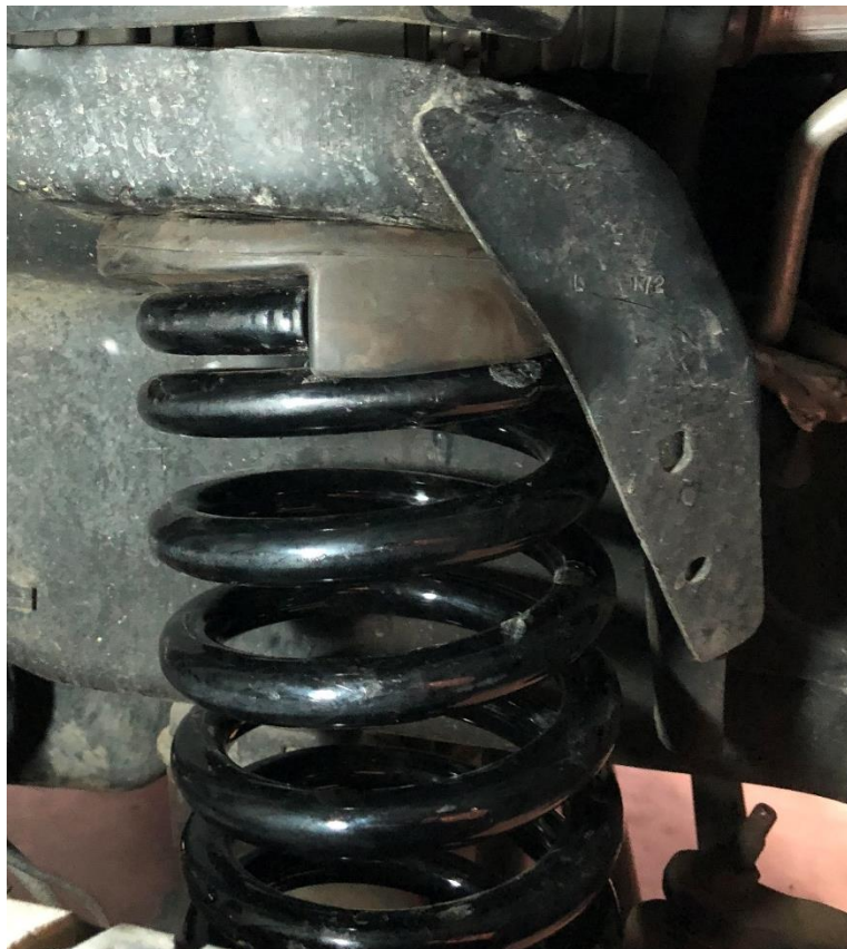
Figure 3. Synergy Leveling Spring Installed, Upper Spring Isolator Correctly Seated
