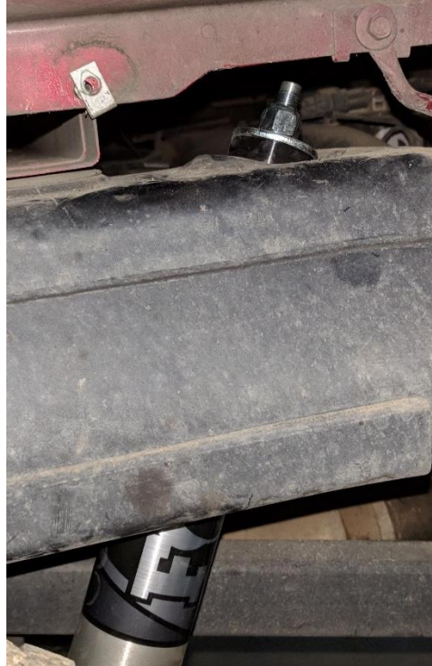
Figure 6. Completed 2500 Rear Shock Installation (Fender Liners Not Installed)
