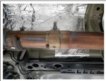
**Step 1.** To remove the OEM exhaust system loosen the clamp fastening the inlet pipe to the Catalytic Converter outlet. Working front to rear disengage all welded hangers from the rubber insulators and remove the system. Do not discard the or damage the rubber insulators as they will be used to mount the new system.
