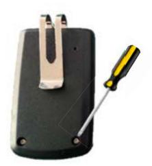
Remove the two screws on the back of the wireless-controller with a Phillips screwdriver to access the batteries
