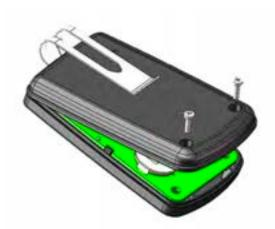
Re-install the back cover to the wireless-controller and tighten the screws with screwdriver. Do not over tighten the screws.
