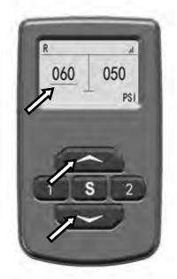
Confirm CH-1/CH-2 on the screen to confirm whether the current status is Channel 1 or Channel 2. The status shown in the figure is Channel 1 in the status shown in the figure.
