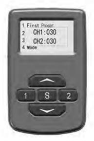
On the First Preset interface, Press and key to change the Preset PSI, and Press and key to change the CH1/CH2.
