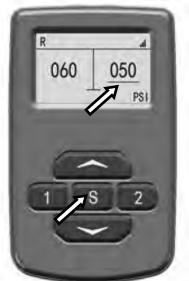
Press the switch from Channel 1 to Channel 2 as shown in the figure.
