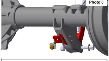
Install Magneride shock relocation brackets.
