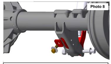
Install Magneride shock relocation brackets.
