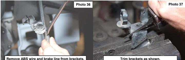
Remove ABS wire and brake line from brackets.
