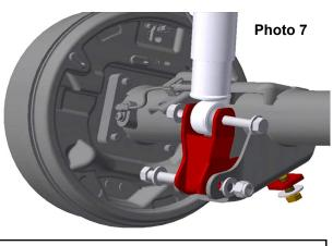
Install Magneride shock relocation brackets.
