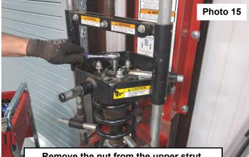
Remove the nut from the upper strut.
