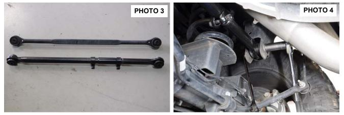
A NOTICE Make sure the adjustment collar/clamps are orientated in the down position to keep from making contact with anything.
