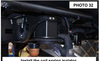
Install the coil spring isolator.
