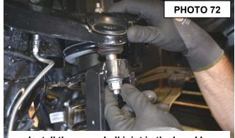
Install the upper ball joint in the knuckle.
