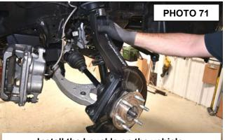
Install the knuckle on the vehicle.
