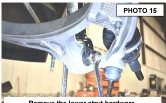
Remove the lower strut hardware.
