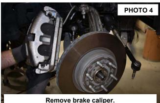
Remove brake caliper bolts.
