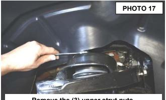
Remove the (3) upper strut nuts.
