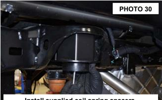
Install supplied coil spring spacers.
