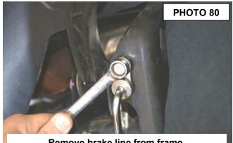
Remove brake line from frame.
