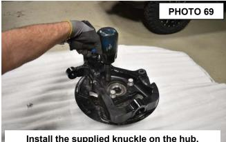
Install the supplied knuckle on the hub.
