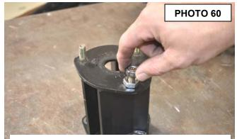
Install the studs in the strut spacer.
