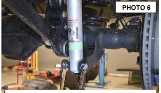
Remove lower shock hardware and shock.
