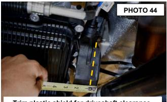
Trim plastic shield for driveshaft clearance.
