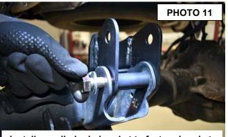
Install supplied relo bracket to factory bracket.
