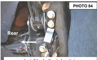
Install brake line in bracket.
