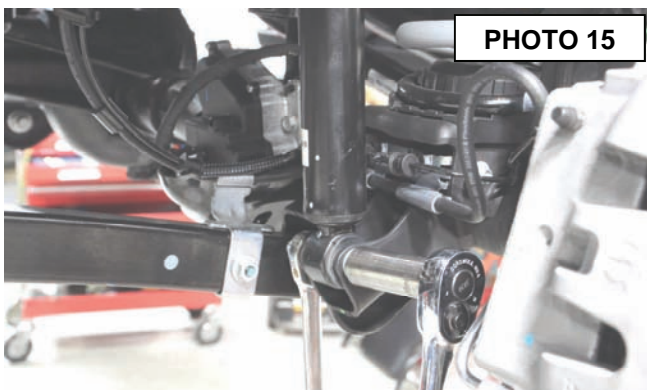
Tighten the lower mounting bolt.
