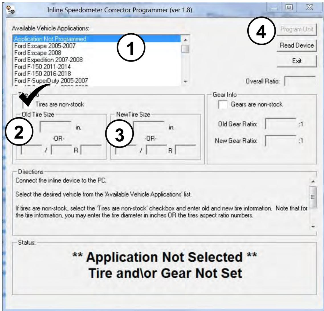
2. For accurate readings, measure the stock and new tire height from the ground to the top of the tire. Enter these measurements (in inches) into the configuration software, and click program to commit these settings. Once configuration is complete, take the Speedometer Calibrator module and harness to the vehicle.
