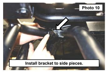
Install the bracket to the top of the cage using the supplied 8mm button head bolts. See Photo 11 and Photo 12.
