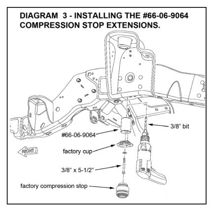
compression stop cup mounting hole in the bottom of the frame to 3/8". Also drill out the hole in the factory cups to 3/8".
