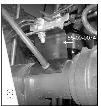
from the other end of the axle and then install the blocks and supplied U-bolts.
