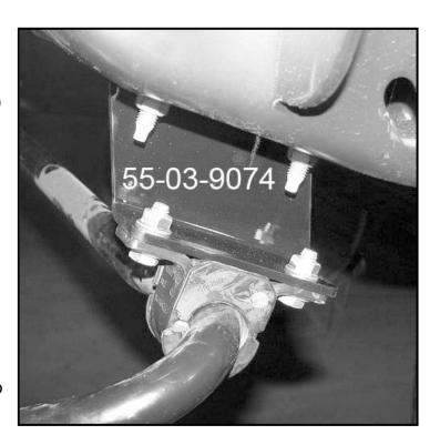
**26)** □□ **FINAL FRONT CLEARANCE and TORQUE CHECK...** Raise vehicle, remove jack stands and lower vehicle to the floor. Cycle steering lock-to-lock and inspect the tires / wheels, and the steering, suspension, and brake systems for proper operation, tightness, and adequate clearance.
