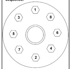
[DIAGRAM 1] to minimize runout. The lug nuts are fully tightened in a later step.
