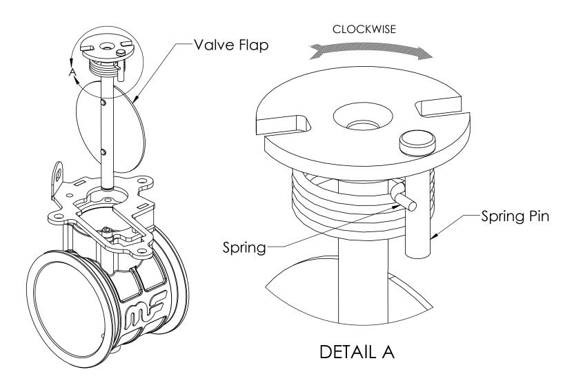
Before installing the OE Valve Motor to the MagnaFlow valve it is very important to have the valve flap oriented correctly.
