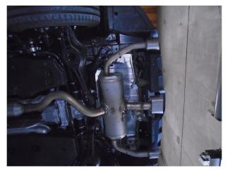
**Step 1:** To remove the OE exhaust begin by unplugging the valve motor at the center tailpipe then un-fasten the hardware at the flange. While supporting the exhaust extract the hangers from the rubber insulators (retain the fasteners and rubber insulators as they will be re-used).
