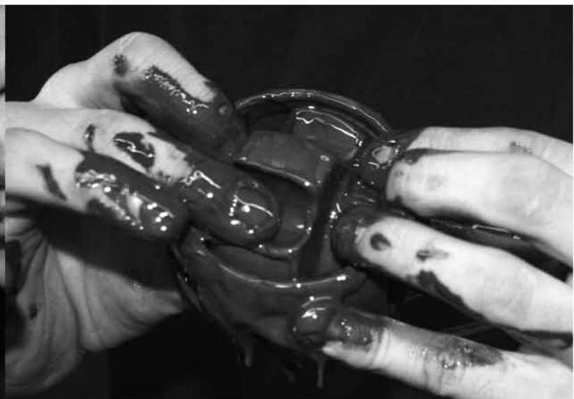
12. Separate the star from the cage by aligning the star into the cage windows. One side of the CV cage is larger for this reason.
