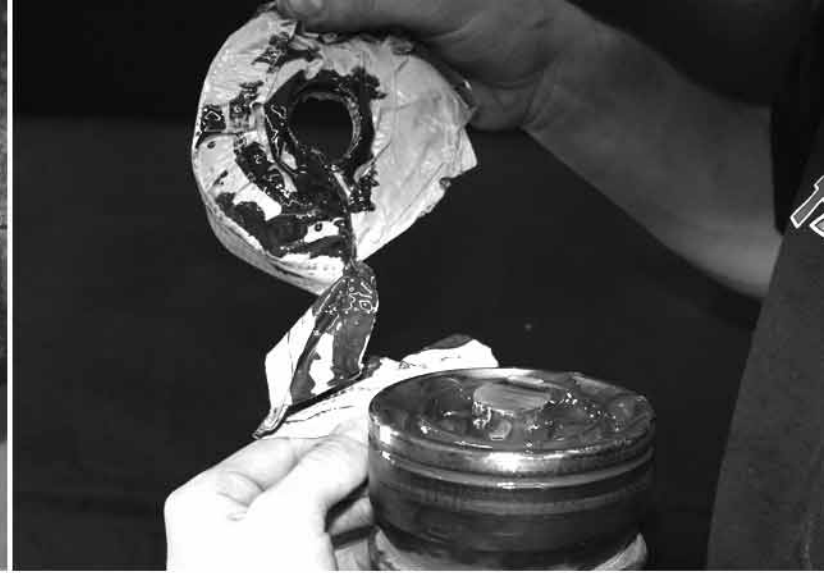
8. Discard the axle and remove the duct tape from the joint.
