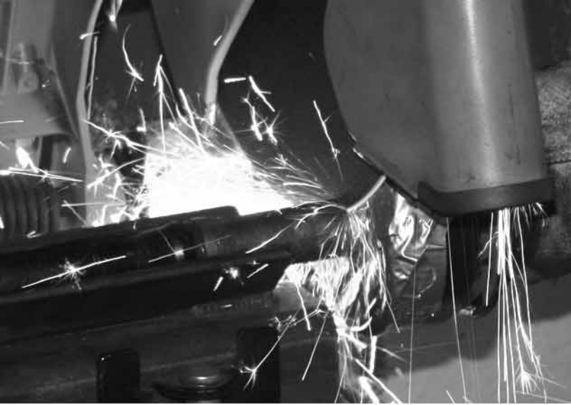
7. Place the axle assembly on the chop saw and cut the axle as close to the joint as possible.
