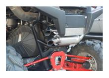
6. Install Item #A slide the hangers in factory mounts from the passenger side until lined up with the header. Once you have it lined up re install the
