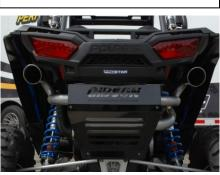
beauty plate. Use the factory bolts and supplied nylock nuts for the top two holes. Once they have been installed tighten the Gibson brackets at the rzr frame. Adjust plate for a level finish.
