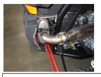
2. Once you have removed the heat shield loosen the factory brackets. Keep loose until final install.
