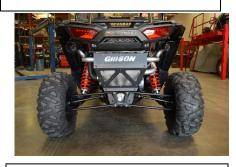
6. Install rear Gibson beauty plate. Use the factory bolts and supplied nylock nuts for the top two holes. Once they have been installed tighten the Gibson brackets at the rzr frame. Adjust plate for a level finish.
