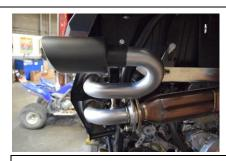
4. Next install the Gibson Muffler assembly. Install the top hanger mounts first then slide the inlet over the factory head pipe re using the factory gasket and bolts. Note: you will relocate the Bolt springs in-between the 2 flanges.
