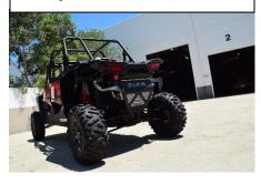
7. Once everything has been installed and tighten install your supplied Gibson tips. Slide the tips on to your desired look and tighten down. Check for 1" clearance and go have fun.
