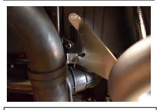
5. Bolt the tailpipe brackets to the rear under bed bracket. You will use Bolt Kit # B. Use the large fender washers on the back side of the top hole. You may have to loosen the factory bracket to adjust for fitment. Do not tighten until all bolts are installed. Install both sides.
