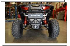
6. Install rear Gibson beauty plate. Use the factory bolts and supplied nylock nuts for the top two holes. Once they have been installed tighten the Gibson brackets at the rzr frame. Adjust plate for a level finish.
