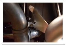
5. Bolt the tailpipe brackets to the rear under bed bracket. You will use Bolt Kit # B. Use the large fender washers on the back side of the top hole. You may have to loosen the factory bracket to adjust for fitment. Do not tighten until all bolts are installed. Install both sides.
