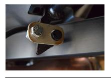
3. Next, Install the supplied bed-lock hardware(Items C and D) Note: Both brackets are to be installed on the same side of the vehicle on either side of the latch. First, tilt open the bed slightly to allow for first bracket to slide over latch post. Then close bed and slide the second bracket over the same latch post securing it with the supplied bolt kit.
