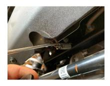
1. To remove the factory muffler, start by removing the retaining spring located on the underside of the muffler followed by the two head-pipe bolts.
