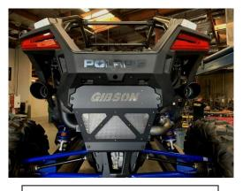
6. Install rear Gibson beauty plate to the upper and lower aluminum exhaust shield brackets re-using the factory hardware and make tight.
