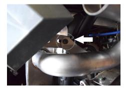
5. Install and fully tighten the nuts on the 3bolt flange and then fully tighten the two bolts that secure the tailpipe brackets.
