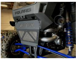
7. Install your Gibson exhaust tips. Slide the tips onto each tailpipe and tighten down with the bolt kit. Be sure to slide them on all the way to make contact with the spark arrestor rivets.
