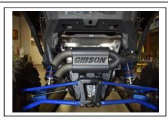
3. Next, install the Gibson Muffler assembly by sliding the two hangers on the muffler into the rubber isolators in the frame while also aligning the three exhaust studs from the turbo headpipe into the three bolt flange. Re-use the factory nuts with anti-seize on the threads and fully tighten.
