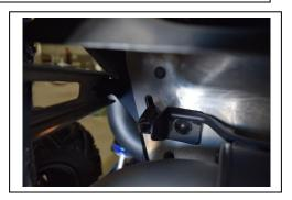
**4.** Re-install the factory upper spring into its original location and attach to the spring hole on the muffler assembly.
