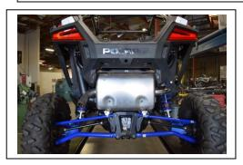
2. Remove the factory exhaust by un-bolting the factory rear shield that covers the muffler. You will re-use the hardware for the Gibson install. Disconnect the 2 factory springs and unbolt the factory exhaust. Do not damage the factory exhaust gasket. You will re-use this gasket. Remove both lower aluminum brackets that hold the factory exhaust shield. They will not be used with this kit.
