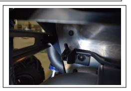
**4.** Re-install the factory upper spring into its original location and attach to the spring hole on the muffler assembly.
