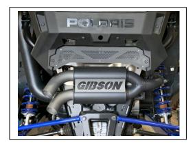
**5.** Lastly, install your new Gibson Beauty Plate onto the upper holes in the rear plastic bumper using the factory hardware as shown in picture. Re-check all hardware for tightness and enjoy the Gibson experience.
