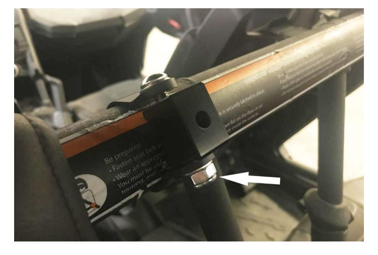
Install the Pivot Bodies (H) with the Screws (I), Washers (F), and Locknuts (J). Snug the straps up, but do not fully tighten, leave the straps loose enough so they can be slid side to side and rotated. Tools Needed: 13mm Wrench, 5mm Hex Key.
