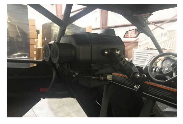
Determine where you want to mount the Helmet Particle Separator. The intake can face forwards or backwards, but it needs to be mounted horizontally, with the Exhaust Fan pointing straight down. It is recommended to mount the Helmet PS in an orientation where there is less dust entering the vortex separators. Also note the Fan Speed Knob is between the Helmet Ports
