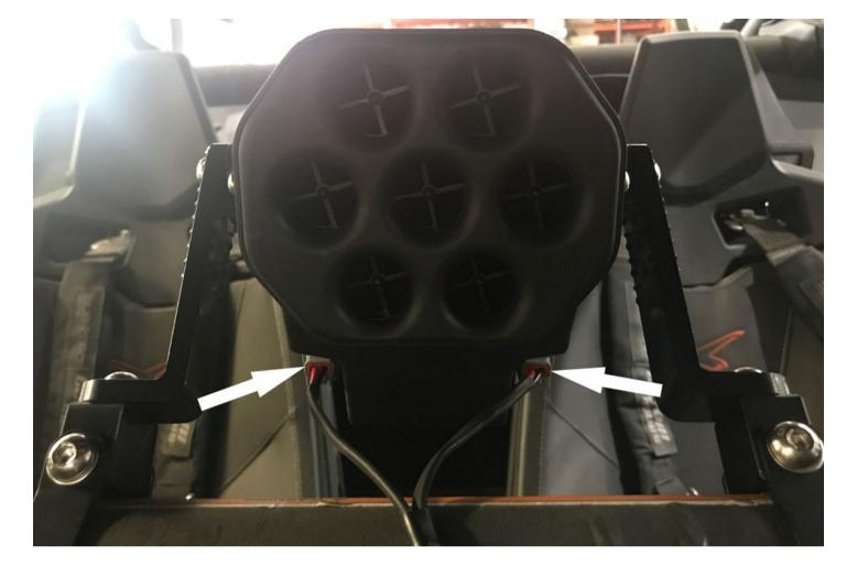
Route the Fan Connectors up to the particle separator and plug them in. There are 2 fans in the Helmet Particle Separator, the scavenge fan that separates the dust, and the blower fan that forces fresh air into your helmet, the connectors are identical.
