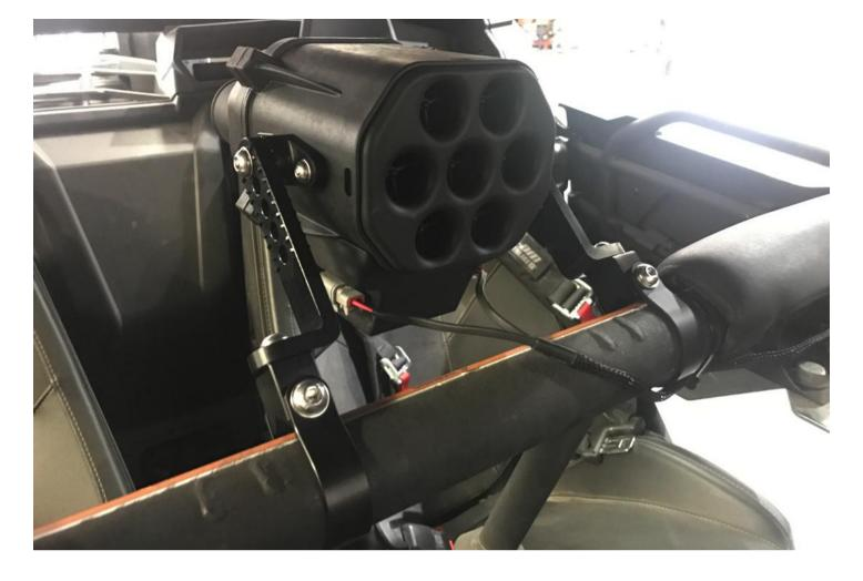
Double check to make sure all connectors are plugged in and secured. Turn the ignition and switch on and make sure air is blowing out the blower and exhaust ports of the Particle Separator. If the exhaust fan does not turn on, double check your electrical wiring. Your installation is now complete. Enjoy your new Helmet Particle Separator.
