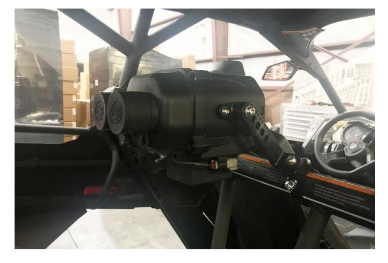
Once you are satisfied with the position of the Particle Separator, tighten the Straps, double check that all mounting screws and nuts are tight and that they are securely mounting the Particle Separator on the roll cage. Tools Needed: 13mm Wrench, 5mm Hex Key.
