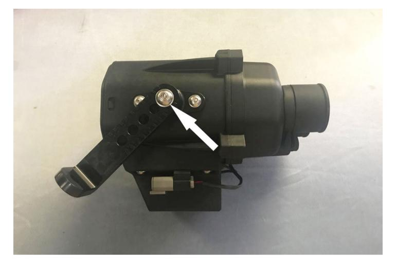
Install the L Brackets (E) onto the Adapters with the Screws (G), Washers (F), and Thread Locker (O), selecting the proper angle and orientation based on the desired location for the Particle Separator, then tighten. Tool Needed: 5mm Hex Key
