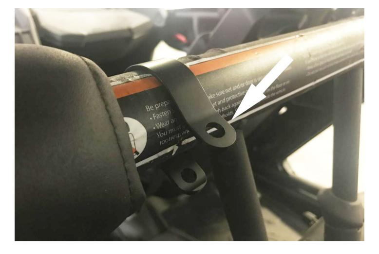
Slide the bar mount straps over roll cage. Wrapping a small parts bag around the roll cage will make sliding the strap over the roll cage easier and help protect the roll cage from scratches.
