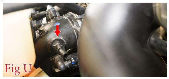
22. Unplug the MAP sensor connector on the tube coming off your throttle body. Also, remove the plastic clip holding the sensor harness to this same pipe. (Fig  $\rm V$ )
