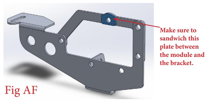
32. IF YOU DO NOT PLAN TO RELOCATE YOUR ADAPTIVE CRUISE CONTROL MODULE, PLEASE SKIP THIS STEP. Mount your adaptive cruise control module/bracket assembly to the intercooler. Use a 13mm Socket & Wrench along with the supplied M8 Bolts (x2), M8 Washers (x3), and M8 Lock Nut (x1). First, position the adaptive cruise module so that it is completely straight with the intercooler. Then, point it slightly towards the sky and tighten both mounting bolts. (Fig AG)
