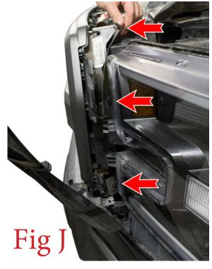
11. Lift the grille up and off the vehicle. There are a couple of clips that hold the front wiring harness to the grille that need to be removed as the grille is being pulled off. (Fig K)
