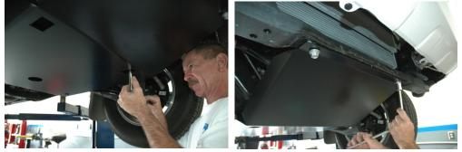
4. Now mount the Transmission Skid Plate to the rear of the IFS Skid and to the crossmember as pictured below using the supplied hardware:
