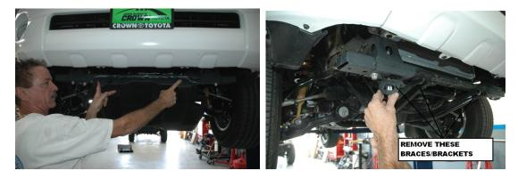
3. Install the All-Pro IFS Skid Plate in place of the factory skid plate using the factory hardware as shown below:
