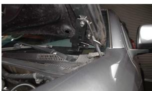
**3.** Remove the lower (rear) hood mounting bolt. Rotate the bracket so the rear hole is aligned with the hole in the hood. Reinstall the hood mounting bolt. Do not fully tighten this bolt yet.
