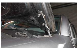
**4.** With the hood mounting bolts loose, slide the bracket forward or rearward as needed to give enough clearance between the bracket and the hood. After enough clearance is achieved, align the marks made on the hood and the hood mounting brackets. Tighten down the hood mounting bolts.
