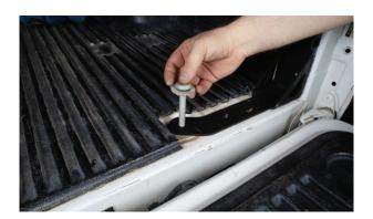
5. Reinstall the bed mount bolt. Once the bed mount bolt is installed push the bottom of the bracket against the side of the bed to take up any space between the two. Snug the bed mount bolt but do not fully tighten it yet. At this point it would be a good idea to raise and lower your tailgate to ensure that the bracket will not interfere with your tailgate. If the bracket prevents your tailgate from closing rotate the bed side of the bracket toward the cab of the truck and retest.
