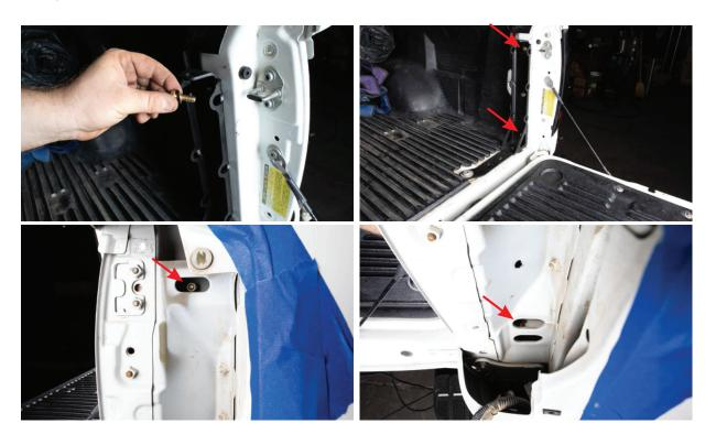
**9.** Install the provided longer 5/16 bolt with a lock washer between the head of the bolt and the flat washer in the location shown. Align the bent bracket on the other side of the bed with the longer 5/16 bolt and tighten the 5/16 bolt. Torque the longer 5/16 bolt to 12 ft/lb MAX.
