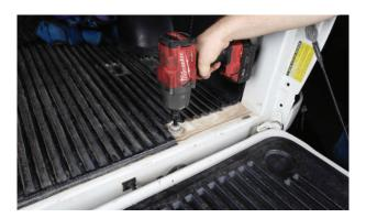
**4.** Set the new bracket in place and align the large bottom mounting hole in the bracket with the bed mount hole in the bottom of the bed. Note the brackets are side specific, with the bracket's bottom curved section oriented toward the front of the vehicle.
