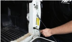
**2.** Remove the taillight and let it hang by the wires. Use care to remove the tail light straight out from the body to avoid damaging the snaps that hold the front of the tail light in place.
