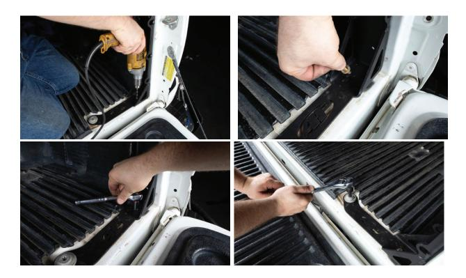
**7.** Using the three holes in the side of the bracket as a guide and a 5/16" drill bit, drill through the side of the bed. Start with the bottom hole and work your way up towards the top of the bracket. Before drilling the next hole make sure that the previous holes in the bed are still aligned with the holes in the bracket.
