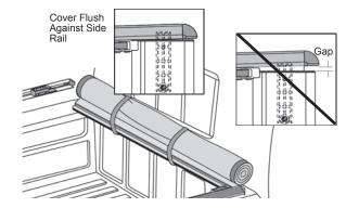
of each Side Rail, with the inside edge of the front bulkhead. Front of Bed Edge of Side Rail Tailgate must align with Inside Edge of Bed
