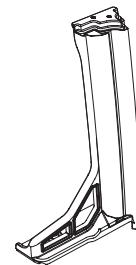
Lower Door Rail Part #577.08 - Right (shown) Part #577.09 - Left Qty. 1 of each
