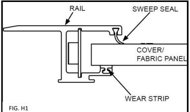
Ensure proper placement of the sweep seal as shown in step 7. Re-apply protectant/lubricant if the cover begins squeaking or sticking during use. *(FIG. H1)*
