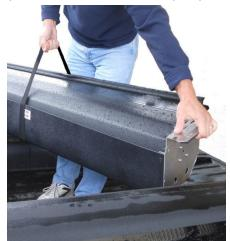
Place the Canister in the truck bed just behind the cab and center it from side to side. Ensuring that the canister is centered in the bed will help assemble the rails to the canister in the next step.
