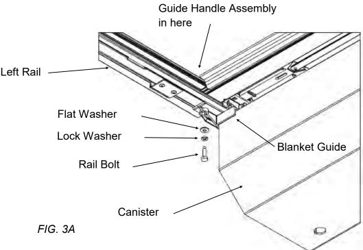
Remove the protective paper from the foam on the underside of the Rail flanges. This is for
