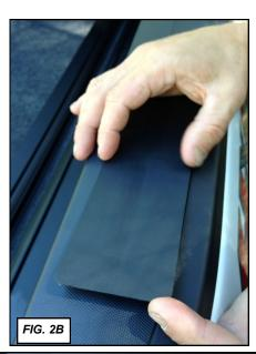
Included with your tonneau cover is a stake pocket cover. This helps to trim the outside seal for your rails (FIG. 2C). First clean the stake pocket hole area. If you have Isopropyl Alcohol this will work well. After the stake pocket area is dry peel off the adhesive backing and stick the cover on the hole so that it is entirely covered (FIG 2A &2B).
