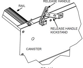
kickstand and lower the release handle. With the handle released the cover will move a short distance and the cover will then lock itself in place. (Cover may not lock tightly against tailgate) This process will allow you to use the cover until power is restored. It is not meant for extended or permanent use.
