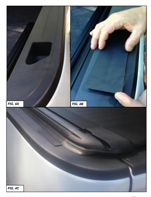
Included with your tonneau cover is a stake pocket cover. This helps to trim the outside seal for your rails (FIG. 4C). First clean the stake pocket hole area. If you have Isopropyl Alcohol this will work well. After the stake pocket area is dry peel off the adhesive backing and stick the cover on the hole so that it is entirely covered (FIG 4A & 4B).
