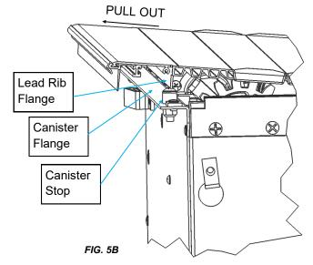
Figure 5B shows that the lead rib needs to be pulled out toward the tail gate. Now hook the rail into the rail guide and roll it down making sure to not get the sweep seal folded back into the rail (FIG 5C &11A).
