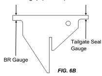
Another way to set the tailgate cap seals is to use the Tailgate Seal Gauge as shown in figure 6B & 6C. You should be able to just slide the Tailgate Seal Gauge in between the Tailgate Cap Seal and the Bottom Cap.
