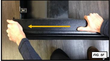
Then you can thread the Lead Rib into the rail an push the rail forward to the end of the can (FIG 5E &5F). If you have difficulty threading the Lead Rib into the rail, you can gently lift up on the lead rib with your left hand while pushing the rail forward with your right. Next push the cab caps into the front of the rails (FIG 5G). Finally secure the rail to the canister with the Rail Screws proved with flat washer and lock washer (FIG 5H).
