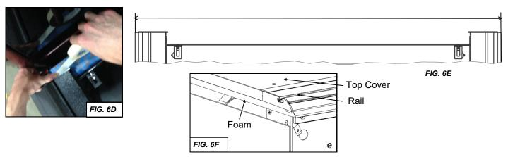
Next mark where the front of the rails sit and mark this position with masking tape, this will be a guide for placing your foam. (FIG 6D). Now pull the cover back until there is room to apply the foam. Lay the foam on the front sill of the truck from rail to rail, trimming the excess with a utility knife (FIG 6E).
