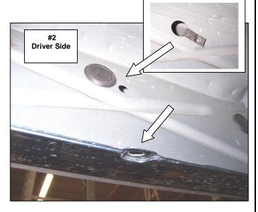
**Step-2** Attach one of the driver side brackets to the rocker panel using the U-Nut, (1) M8 hex bolt, (1) 5/16" lock washer and (1) 5/16" flat washer, and to the pinch mold using (1) M8 hex bolt, (2) 5/16" flat washers, (1) 5/16" lock washer, and (1) M8 hex nut. Leave the nut and bolts loose for final adjustment, **(Photo 3)**.
