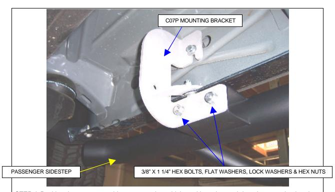
**STEP-6** Position the passenger sidestep up to the vehicle and loosely attach it to the mounting brackets using the 3/8" x 1 1/4" hex bolts, flat washers, lock washers and hex nuts.
