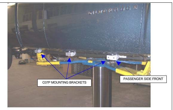
**STEP-5** Locate the holes in the body for the center and rear mounting brackets. Measure rearward from the front fender bolt 37 ¾" for the center and 67" for the rear bracket. Repeat steps 3 & 4 to install the center and rear brackets.
