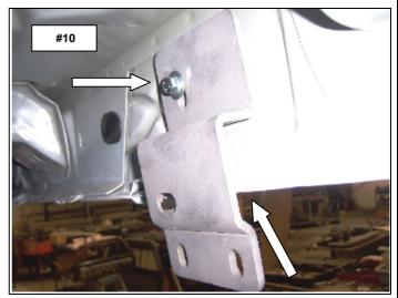
Step-6 Passenger side rear bracket installation.
