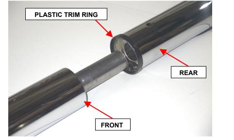
STEP 2. INSTALL THE PLASTIC TRIM RING ON THE REAR SECTION AND INSERT THE FRONT SECTION INTO THE REAR SECTION.
