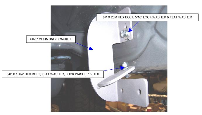
**STEP-3** Loosely attach one of the C07P mounting brackets to the rocker panel and pinch mold using the 8M, 5/16" and 3/8" fasteners as shown.
