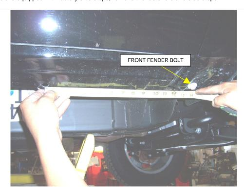
**STEP-2** This installation uses three mounting brackets per side. Begin by installing the passenger side front mounting bracket. Measure rearward from the front fender bolt approximately 14" and locate the single hole in the body pinch mold and the square nut spot welded in the rocker panel.
