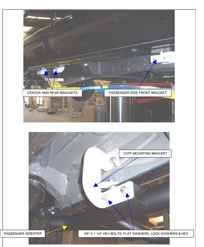
**STEP-6** Position the passenger side step up to the vehicle and loosely attach it to the mounting brackets using the 3/8" x 1 1/4" hex bolts, flat washers, lock washers and hex nuts.
