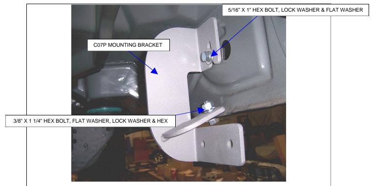
**STEP-5** Loosely attach the two remaining C07P mounting brackets to the rocker panel and pinch mold using the 5/16" and 3/8" fasteners as shown.
