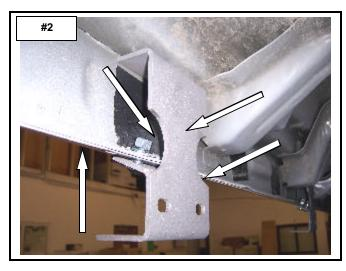
**STEP 2.** ATTACH EACH OF THE MOUNTING BRACKETS TO THE PINCH MOLD USING (2) 3/8" X 1" CARRIAGE BOLTS, (2) FLAT WASHERS, (2) LOCK WASHER AND (2) HEX NUTS. HAND
