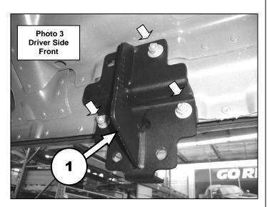
**Step-3** Locate the (3) threaded studs on the inner rocker panel at the rear of the cab and repeat the above steps to install one of the mounting brackets, (Photo 4 & 5).
