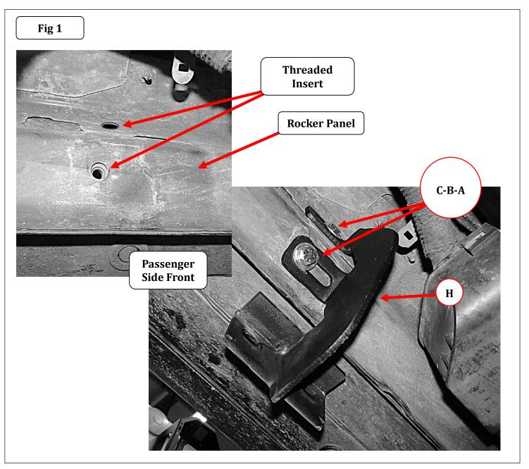
**Step-2** Locate the threaded inserts on the inner rocker panel at the center and rear of the cab and repeat step 1 to install the brackets using the supplied hardware. Note: The front mounting location is shown in Figure 2. The center and rear mounting locations are similar.
