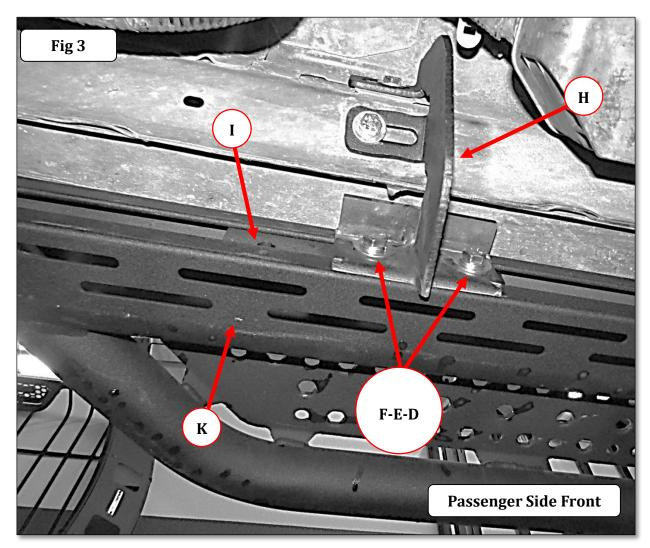
**Step-5** Tighten the nuts securing the brackets to the rocker panel and the bolts securing the Dominator D6 running board to the brackets.
