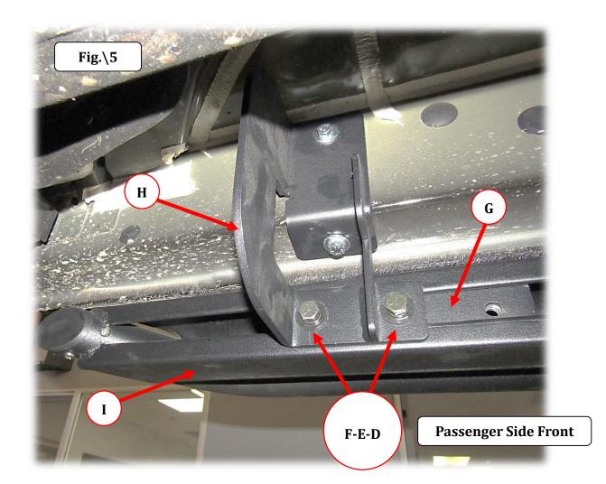
**Step-6**Tighten the bolts securing the mounting brackets to the body panel and the bolts securing the Dominator DSS side step to the mounting brackets.
