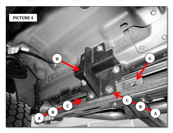
**Step-5** Align the Dominator DSS side step with the vehicle and tighten all bracket and side step nuts and bolts,. Repeat the above steps to install the driver side brackets and Dominator DSS side step.
