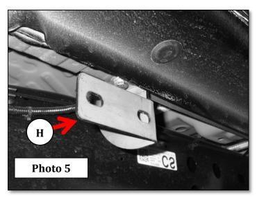
**Step-5** Insert four of the Nut-Plates through the rectangular opening in the back of the Dominator DSS side step. Measure and position each Nut-Plate so it aligns with one of the three mounting brackets previously attached to the vehicle, (Photo 6).
