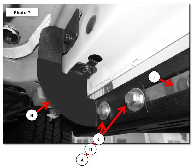
**Step-7** Align the Dominator DSS side step with the vehicle and tighten all bracket and side step nuts and bolts,. Repeat the above steps to install the brackets and Dominator DSS side step on the driver side of the vehicle.
