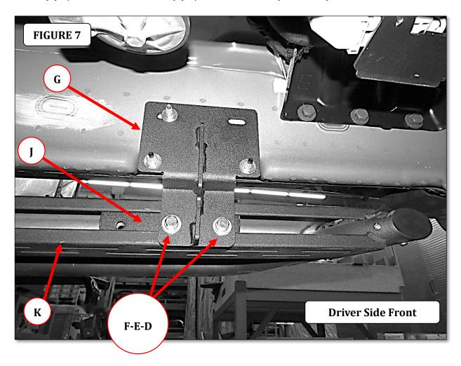
**Step-7** Tighten the nuts securing the brackets to the rocker panel and the bolts securing the Dominator DSS slider step to the brackets.
